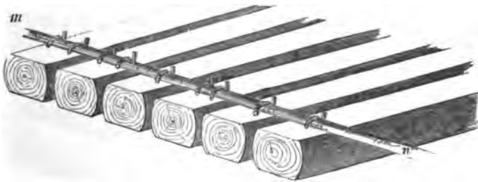
Fig. 273.—Rigid raft-section with pole.
